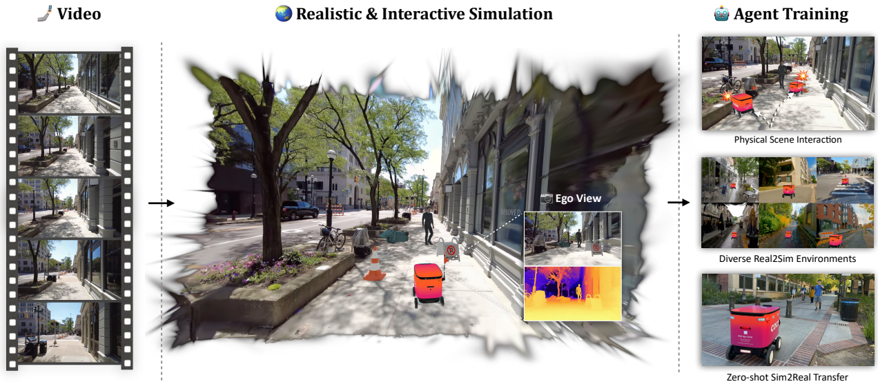
Figure 1. Vid2Sim converts monocular video captured by a hand-held camera into realistic and interactive 3D simulation environments. It facilitates RL training of navigation agents in digital twins of urban scenes and provides realistic observations like RGB and depth to reduce the sim-to-real gap. The pink mobile robot in the image is a food delivery bot that avoids collisions with pedestrians and obstacles.
