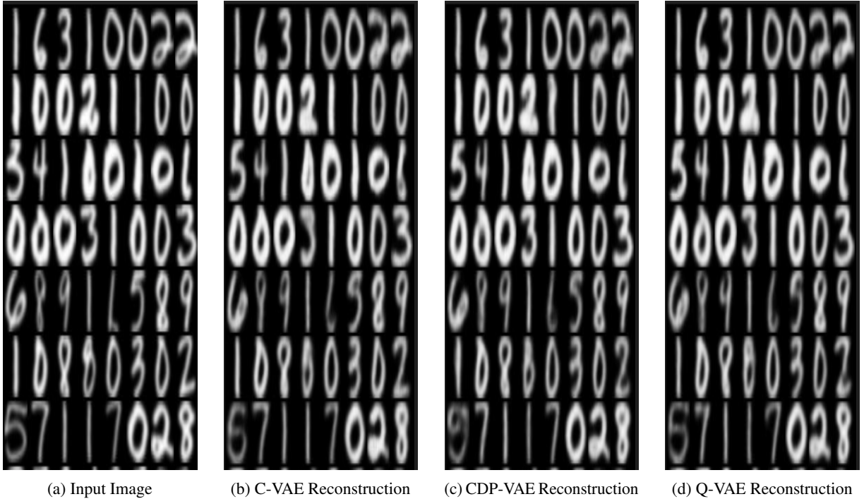
Figure 11: Comparing Classical and Quantum Reconstructed Images. (a) USPS Input Up-sampled Image from 16x16 to 32x32 resolution (b) Classical VAE Image Reconstructions, (c) USPS CDP-VAE reconstructed images and (d) USPS Q-VAE reconstructed images for Variational Autoencoder.
