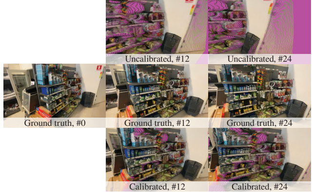
Figure 6. Metric-calibration on DL3DV, frames #12 and #24. Uncalibrated re-projections (top row) deviate significantly from the ground truth (middle row), hindering both the re-projected condition (Section 3.4) and evaluation (Section 4.1). Calibration (bottom row) rectifies this discrepancy.
