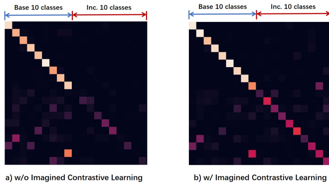
Fig. 6. Confusion matrices of different contrastive losses. The last 10 base classes and the first 10 incremental classes on miniImageNet are zoomed in for ablation comparisons.
