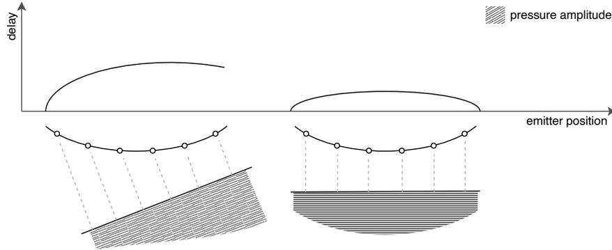
**Fig. 3.** Visualization of two plane wave image transmission event with different angles. The added delays depend on the transmission angle and the transducer geometry. Due to the cosine weighting described in equation 6, we see the change in the amplitude of the pressure over the rays.
