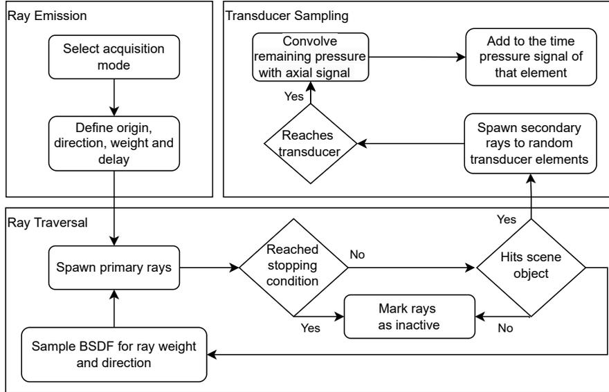
**Fig. 2.** Flow diagram on the main parts of the ray tracing: the ray emission based on the transducer geometry, the ray traversal through the scene, and the transducer sampling to enhance the likelihood of the rays reaching the transducer
