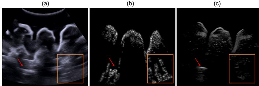
**Fig. 5.** Comparison of (a) real acquisition, (b) baseline simulator, and (c) UltraRay. The orange box highlights unrealistic reflections present in the baseline simulator compared to the real and the proposed method. Additionally, the red arrow showcases a realistic reflection in UltraRay that is also present in the real acquisition while it appears highly distorted in the baseline.
