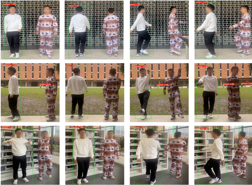
Figure 16: The attack effects are demonstrated in three different scenarios: a hallway, a lawn, and a library. For each scenario, we recorded a video of approximately 1 minute with a frame rate of 30 FPS, using an iPhone 13 as the recording device. The confidence threshold is set as 0.5. The experiment shows that we can successfully fool Faster R-CNN in various scenarios.
