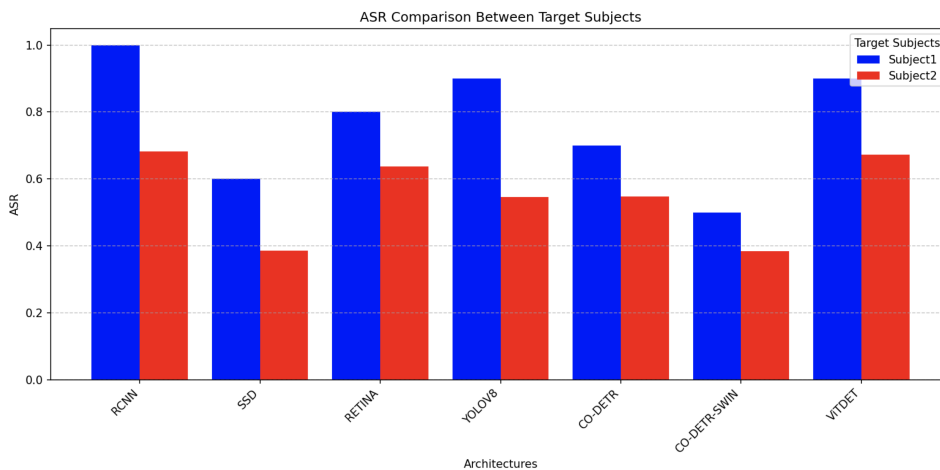
Figure 19: The attack transferability on unseen subjects. We train the adversarial patch on subject 1 and then test the ASR on subject 2. The white-box model is Faster-RCNN. The Y-axis is the attack success rate.
