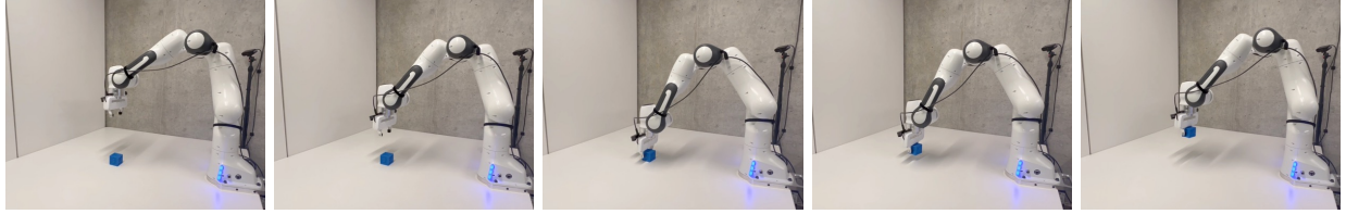
Figure 7 Real-world Deployment: We show an example episode of our policy performing the cube picking task on a Franka robot in the real world. We use Toto -base to run the robot at real time, despite being a small model, Toto was able to achieve about 63% success rate in real world setting.
