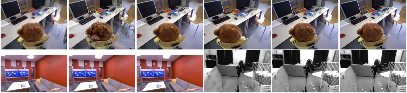
Figure 1. Our method Scaffold-SLAM achieves high-quality photorealistic mapping with quality outperforms state-of-the-art methods (GS-ICP SLAM [1], Photo-SLAM [2], SplaTAM [3], MonoGS [4]) across monocular, stereo, and RGB-D cameras. Top: The results are from TUM RGB-D datasets for RGB-D camera. Bottom: The left three images stemming from Replica datasets for monocular camera and the right three from EuRoC MAV datasets for stereo camera. Non-obvious difference in quality highlighted by insets.
