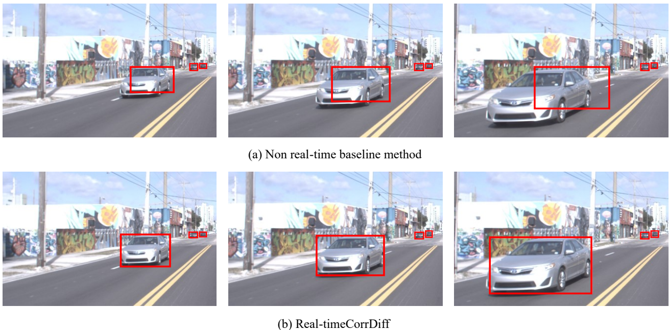
Fig. 7. Demonstration of Non-real-time methods and CorrDiff on the Argoverse-HD dataset under streaming perception settings. Non-real-time methods (a) exhibits large object displacement error for its long communication and computation delay. CorrDiff (b) manages to produce up-to-date results for its low inference time and its ability to adapt to different delays and objects velocities.
