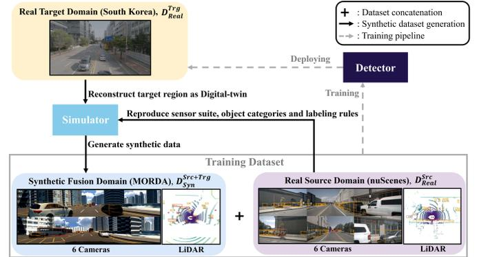
Fig. 1. Research overview: Cost-effective generation of virtual data ( $D_{Syn}^{Src+Trg}$ ) which mimics real-world dataset that one could construct if the sensor configuration of  $D_{Real}^{Src}$  were dispatched to the real-target domain  $D_{Real}^{Trg}$ . The usefulness of our method is assessed by training object detectors on ( $D_{Real}^{Src} + D_{Syn}^{Src+Trg}$ ) and evaluating on unforeseen  $D_{Real}^{Trg}$ .
