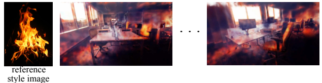
Figure 10. Video stylization results using GaussianVideo. Starting with a ‘fire’ style applied to the first frame, the style is propagated across the video by updating only the SH coefficients, ensuring consistent stylization without additional supervision. The visual coherence across frames highlights GaussianVideo’s ability to maintain high-quality style transfer while preserving structural details throughout the sequence.
