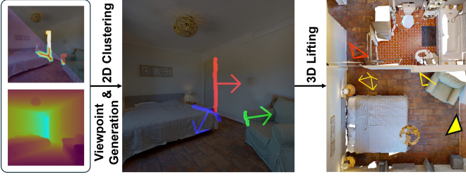
Fig. 5: 3D Frontiers Generation: Each frontier pixel is assigned a 2D viewing angle derived from the depth gradient. Combined with the info gain, 2D clustering is applied to obtain sparse 2D frontier clusters with associated viewing directions (middle). The foreground and background depths near the frontier pixels are then utilized to lift each clustered 2D frontier into 3D space.
