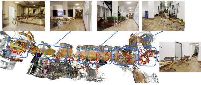
Fig. 11: Exploration process of a quadrupedal robot in a real-world environment. The mapping result is generated through TSDF integration using monocular depth prediction from the onboard RGB camera.
