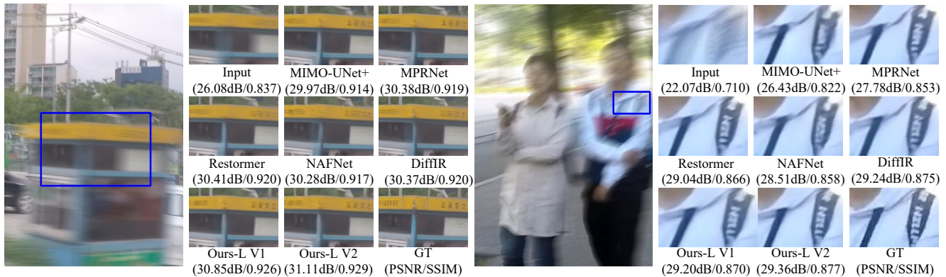
Fig. 11: Image motion deblurring comparison on the images “GOPR0410_11_00-000190” and “55fromGOPR1096.MP4” from GoPro [87] and HIDE [88]. Our MB-TaylorFormer-XL V2 obtains sharper and visually-faithful results.
