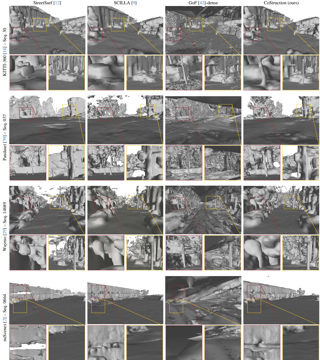
Figure 3. Qualitative experiments results on four popular autonomous driving datasets. Complex scene geometries reconstructed by the mesh are color highlighted. We compare our mesh to the ones from StreetSurf [12], SCILLA [9] and GoF [42]
