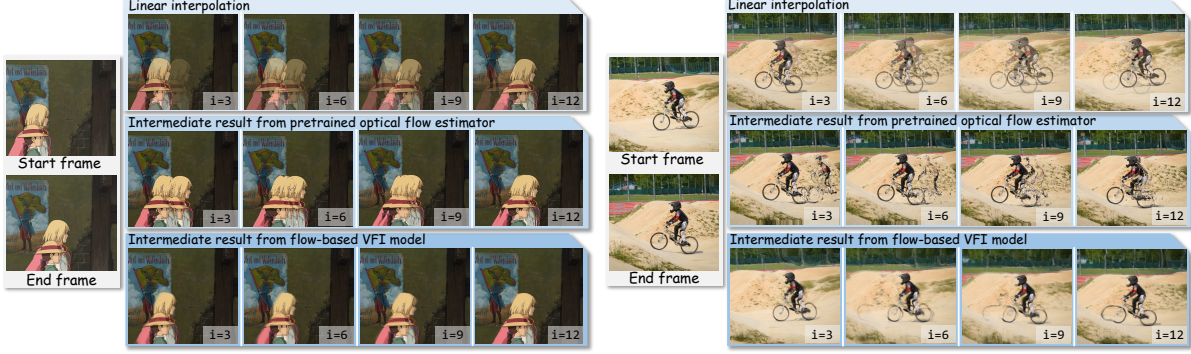
Figure 3. Comparison of different methods for approximating intermediate frames. Linear interpolation merely overlays the input frames, while optical flow often introduces significant artifacts. In contrast, the frames warped through intermediate flow demonstrate superior stability, providing the generative model with robust correspondence information.
