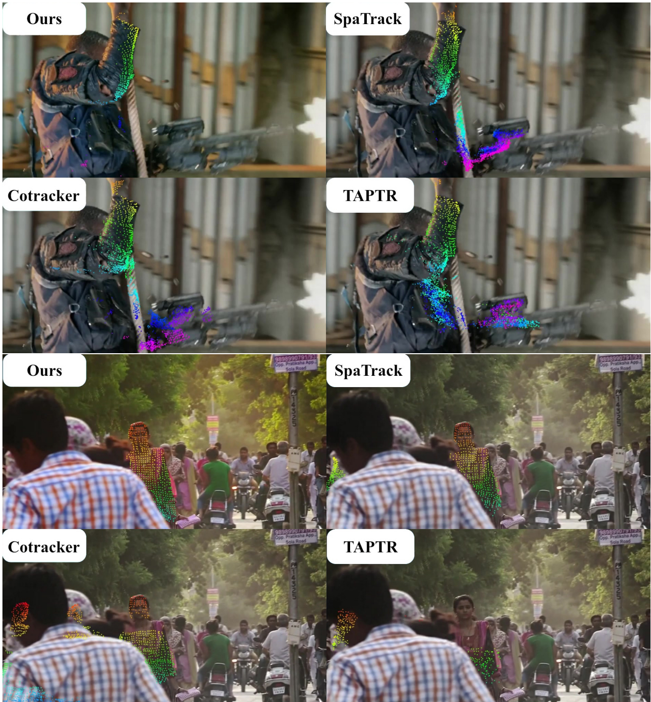
Figure 4. Results of tracking at a higher frame rate. Sliding window based methods can mispredict points to other regions during occlusion (e.g. the gun and rope in shooting and the wrong person in india ), while ours exhibit robustness.
