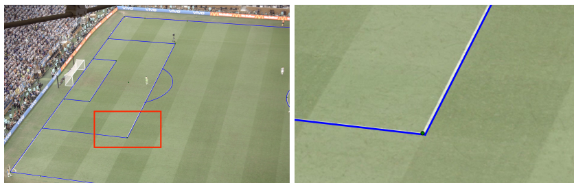
Fig. 7: Visualization of the annotation tools: manual annotation (left) and zoomed-in view (right). The manually selected point is indicated by the green marker. The blue lines show the preview results of the projection using the manually selected points.
