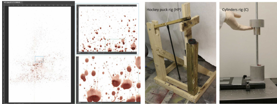
Figure 1: On the right is a sample of impact spatter pattern; the scale is on the edge. The test rigs used for generating the patterns is shown on the left. The figures are taken from [21].
