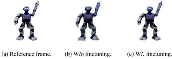
Figure 3. Ablation studies on finetuning the 3D Gaussians in the Initialization stage reveal that finetuning can capture finer texture details in the reference frame, enhancing the quality of subsequent generation.
