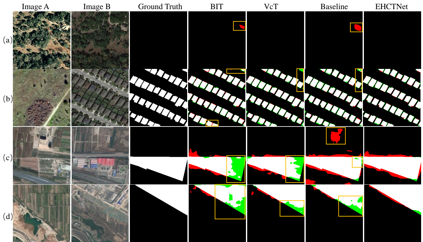
Figure 8. Visualization results of different methods on the LEVIR-CD ((a) and (b)) and DSIFN-CD ((c) and (d)) test datasets. Different colors are utilized to highlight the performance differences among these methods in change detection tasks: white for true positives, black for true negatives, red for false positives, and green for false negatives. The orange rectangle indicates the presence of missed detections, discontinuity, and incorrect merging of adjacent change areas.
