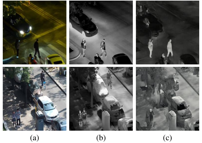
Fig. 2. Comparison of (a) Visible, (b) Ground Truth Infrared, and (c) Generated Infrared images.
