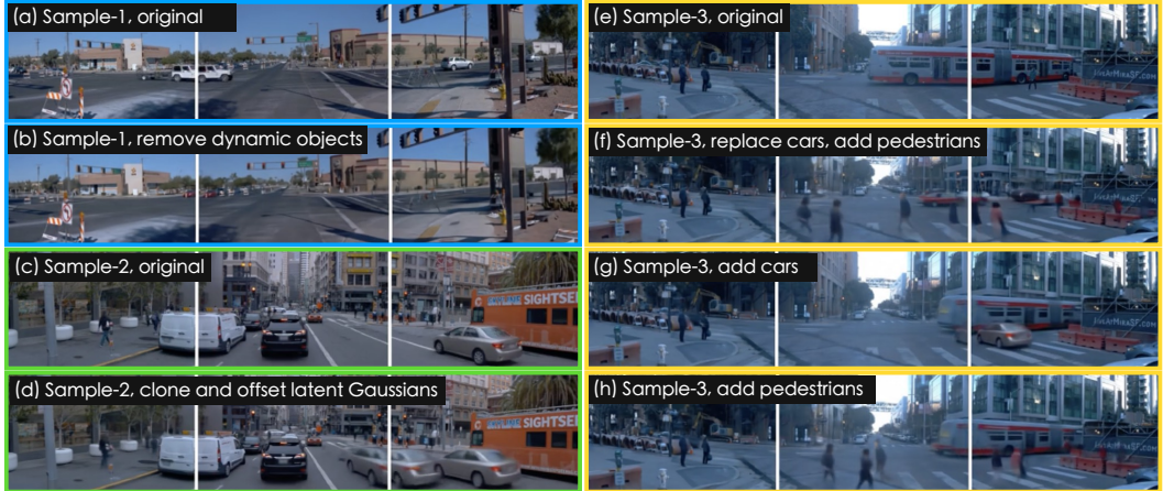
Figure 7: STORM editing examples. We present examples of removing or cloning vehicles (a-d), as well as adding or replacing pedestrians and vehicles (e-h). Notice how STORM harmonizes the edited images due to the use of the decoder. More examples can be found at our project page .
