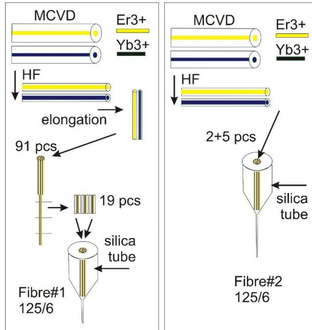
Fig.1 Scheme of fabrication of a)-left nanostructured Er<sup>3+</sup> and Yb<sup>3+</sup>-doped silica fibre (Fibre#1) and b)-right structured core Er<sup>3+</sup> and Yb<sup>3+</sup>-doped silica fibre (Fibre#2).
