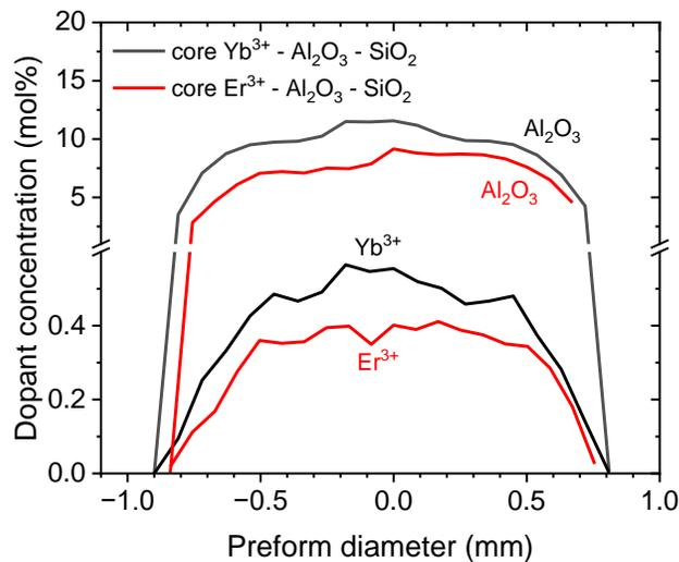
Fig. 4 Distribution of  $\text{Al}_2\text{O}_3$ ,  $\text{Yb}^{3+}$  and  $\text{Er}^{3+}$  dopants in typical initial MCVD preforms determined by EMA.
