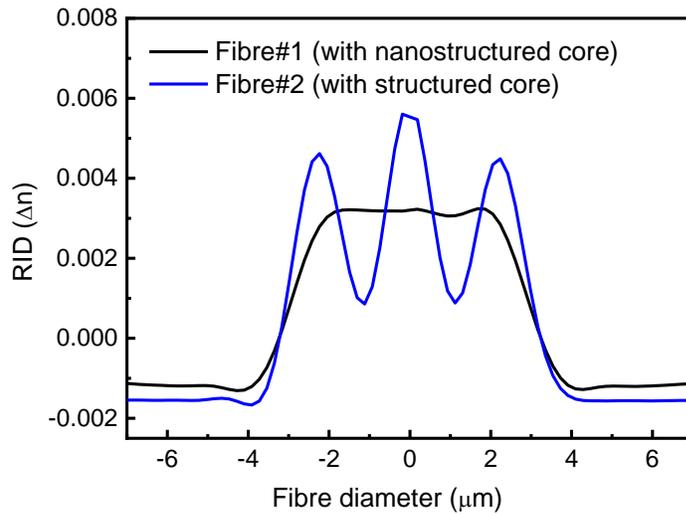
Fig. 5 RIP of  $\text{Er}^{3+}$  and  $\text{Yb}^{3+}$ -doped fibres with nanostructured core (Fibre#1) and structured core (Fibre#2) measured with IFA-100.
