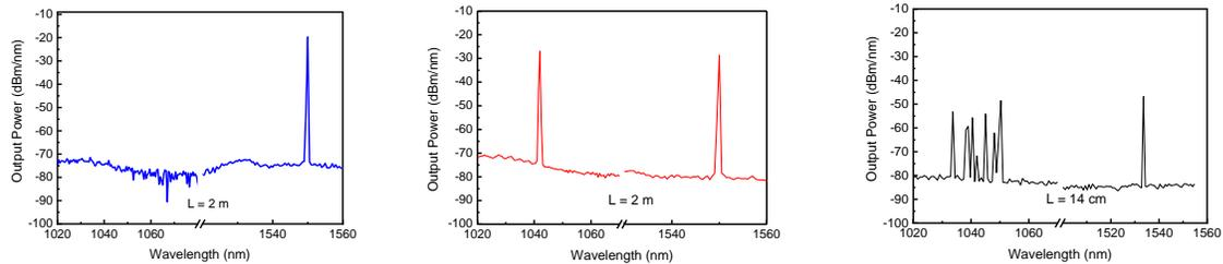
Fig. 9 Laser emission of  $\text{Er}^{3+}$  and  $\text{Yb}^{3+}$ -doped fibres a) Fibre#1 (with nanostructured core), b) Fibre#2 (with structured core), and c) nanostructured phosphate fibre.
