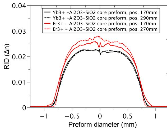
Fig. 3 RIPs of typical initial MCVD preforms doped with  $\text{Yb}^{3+}$  (black) or  $\text{Er}^{3+}$  (red) and  $\text{Al}_2\text{O}_3$  used for structuring, measured at the end and middle of the preforms.
