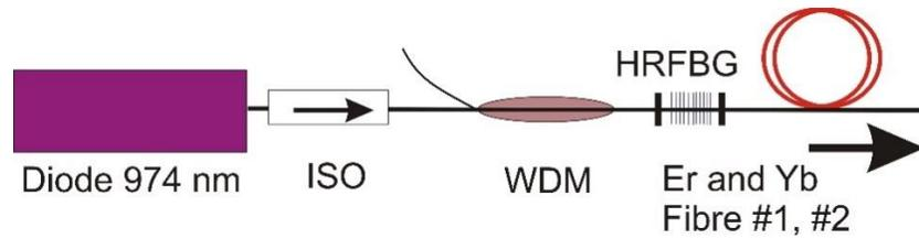
Fig. 2 Fibre laser setup used for characterization.
