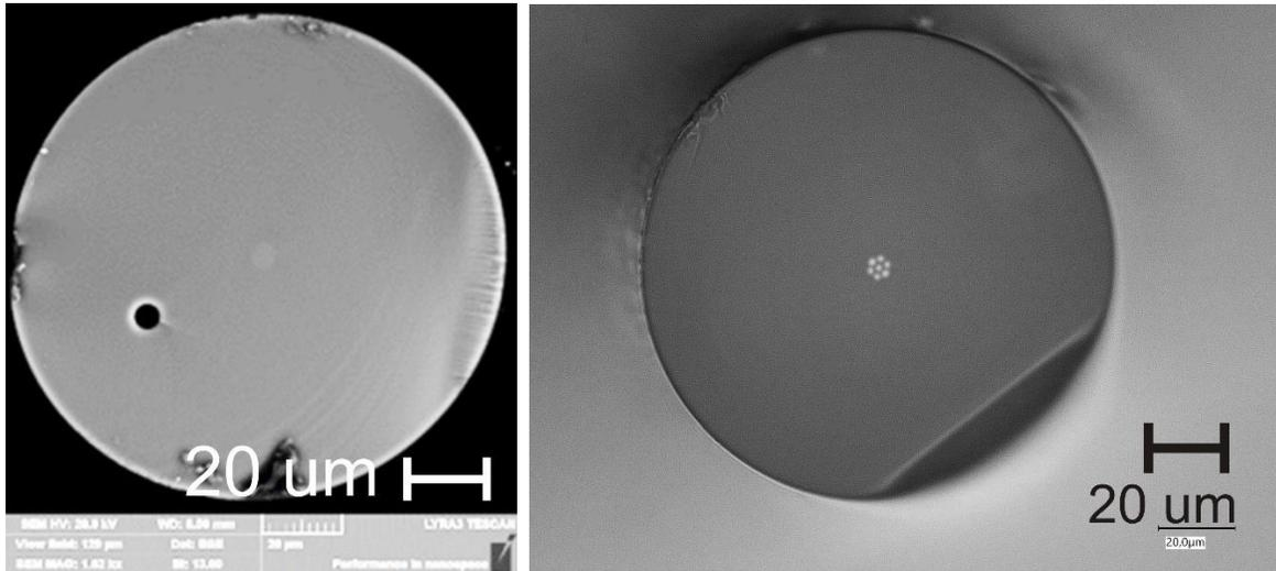
Fig. 6 Cross section of  $\text{Er}^{3+}$  and  $\text{Yb}^{3+}$  doped fibres a) SEM of Fibre#1, core composed from 1729 initial rods, b) Micro photo of Fibre#2, core composed from 7 initial rods.
