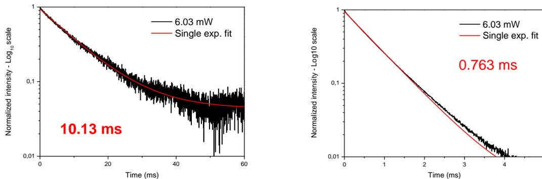
Fig. 8 Fluorescence lifetimes of  $\text{Er}^{3+}$  ions (a) and  $\text{Yb}^{3+}$  ions, (b) embedded in Fibre#1.
