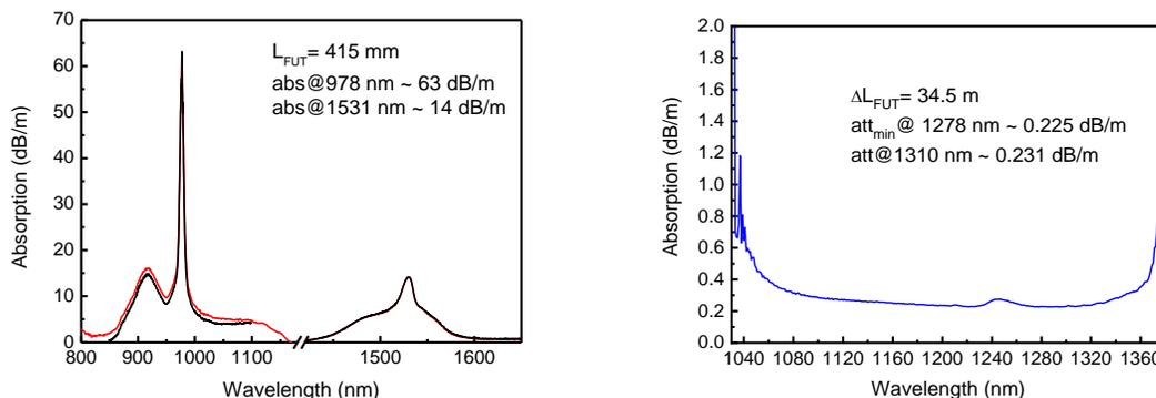
Fig. 7 Optical losses of Fibre#1 a) absorption bands of  $\text{Er}^{3+}$  and  $\text{Yb}^{3+}$ , b) background losses.
