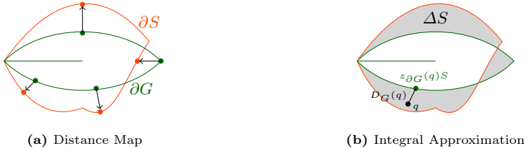
Fig. 3: The boundary of ground truth area G , \partial G , is shown in green and the boundary of segmentation mask S , \partial S is shown in orange.
