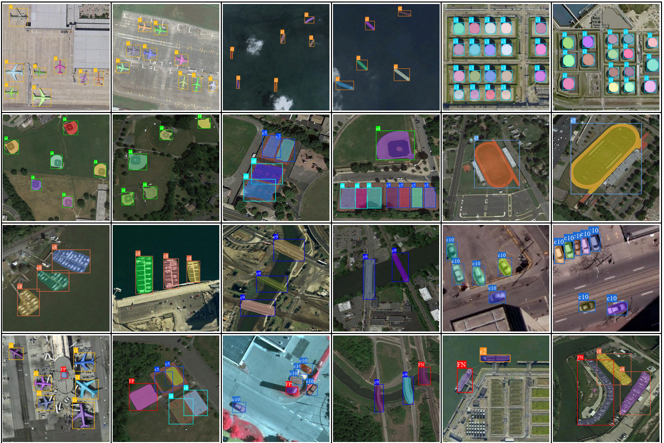
Fig. 13. The instance segmentation results on the NWPU VHR-10 dataset from SG-LRN. The predicted true positive instances are annotated with randomly colored bounding boxes attached with their category texts. The predicted false negative and false positive instances are annotated with red colored bounding boxes attached with the texts "FN" and "FP", respectively.
