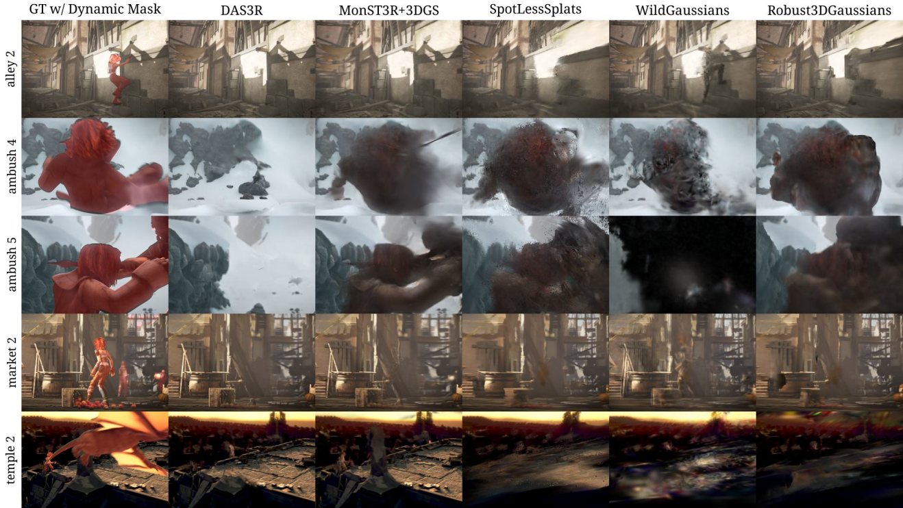
Figure 5. Qualitative comparison on Sintel dataset. DAS3R is robust to large dynamic objects while other methods fail to remove the dynamic objects and even fail to reconstruct the overall scene .
