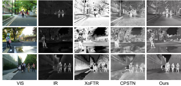
Figure A1. Visualization Results of Infrared generation on MSRS. The first two columns are real RGB and Infrared images.
