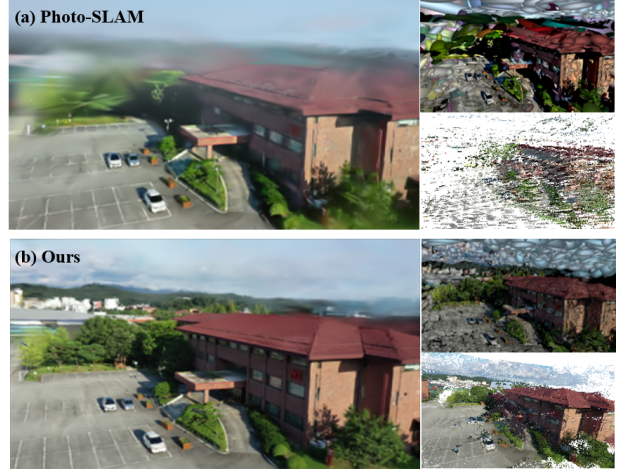
Fig. 1. Rendering results of (a) Photo-SLAM [20] and (b) our method. The optimized Gaussian points and the estimated point cloud for each method are shown in the upper right and lower right, respectively. Our method utilizes an online MVS approach to generate a dense point cloud, which is then used to initialize Gaussian points. As a result, our method produces a 3DGS model with much higher rendering quality compared to Photo-SLAM, which relies on a sparse point cloud.
