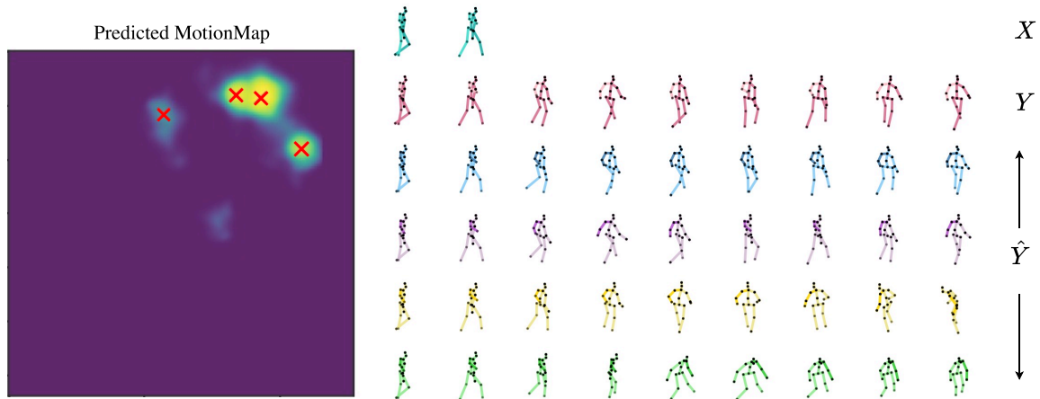
Figure 5. Ranking. Since MotionMap can predict variable number of modes with their associated confidences, our method also allows us to rank predictions. For instance, the highest ranked prediction (top row among \hat{Y} ) closely matches the ground truth motion. However, rare modes (bottom row) are ranked low since the corresponding mode has a lower confidence.
