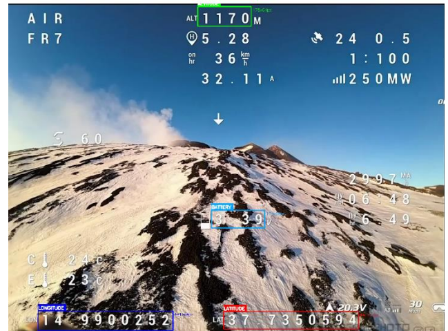
Figure 2. The ROI validation preview window depicts manually labeled ROIs drawn by the user.
