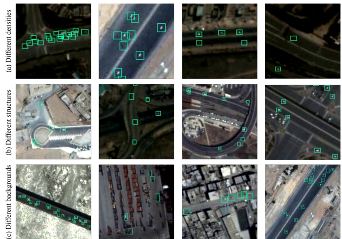
Fig. 2. Example images and their annotations in the SDM-Car dataset. Our dataset shows diversity in terms of instance density, road structure, and background, and contains a large number of dim instances.
