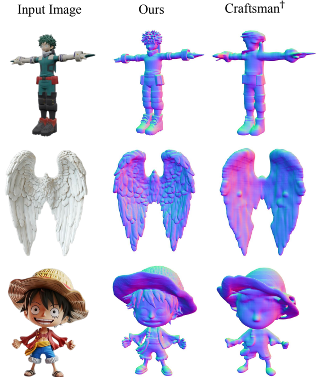
Figure 7. The diffusion results of the single image to 3D generation trained on our Dora-VAE and Craftsman † . The 3D geometry generated by the diffusion model trained on our proposed Dora-VAE has more details under the same experimental environment.
