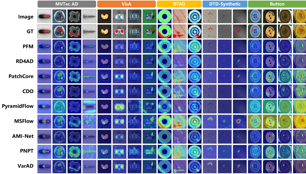
Fig. 3. Anomaly maps on the four publicly available datasets and our private data from the real-world button inspection task.
