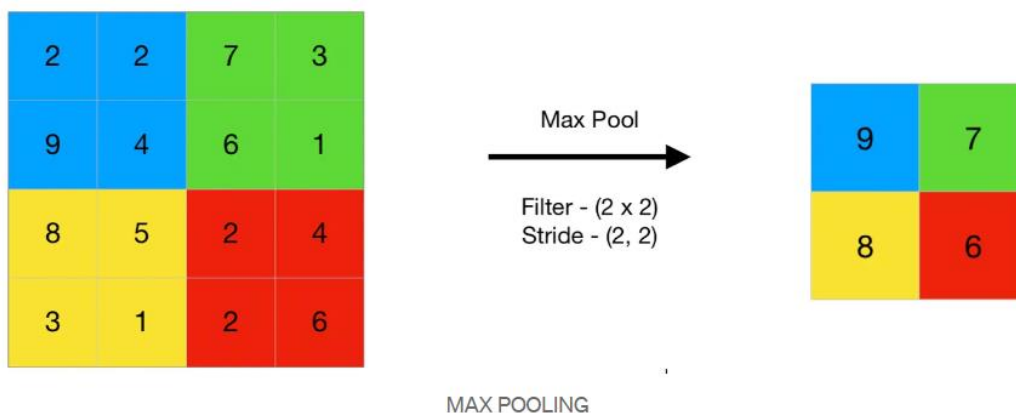
Fig4. This image illustrates the Max Pooling process in neural networks. A 4 \times 4 input matrix is processed using a 2 \times 2 filter with a stride of 2. For each 2 \times 2 block, the maximum value is selected, resulting in a 2 \times 2 output matrix. This operation helps reduce dimensionality while retaining important features of the data.
