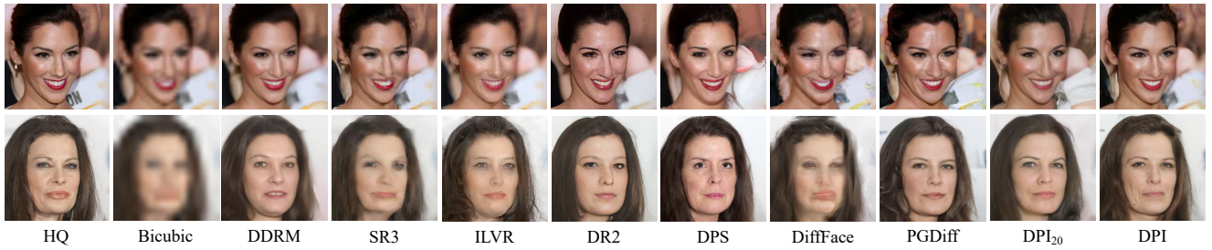
Figure 4: From top to bottom are the FSR results of DPI and DDPM-based methods on CelebA1000 testset at \times 8 , and \times 16 scales, respectively. DPI_{20} refers that the DDIM (Song, Meng, and Ermon 2020) algorithm samples only 20 steps. Please zoom in for best view.
