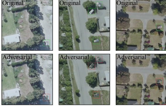
Figure 5. Examples of adversarial images are shown, with the top row displaying the original images and the bottom row showing the corresponding adversarial (T-PixFcMa) images produced using Blender.
