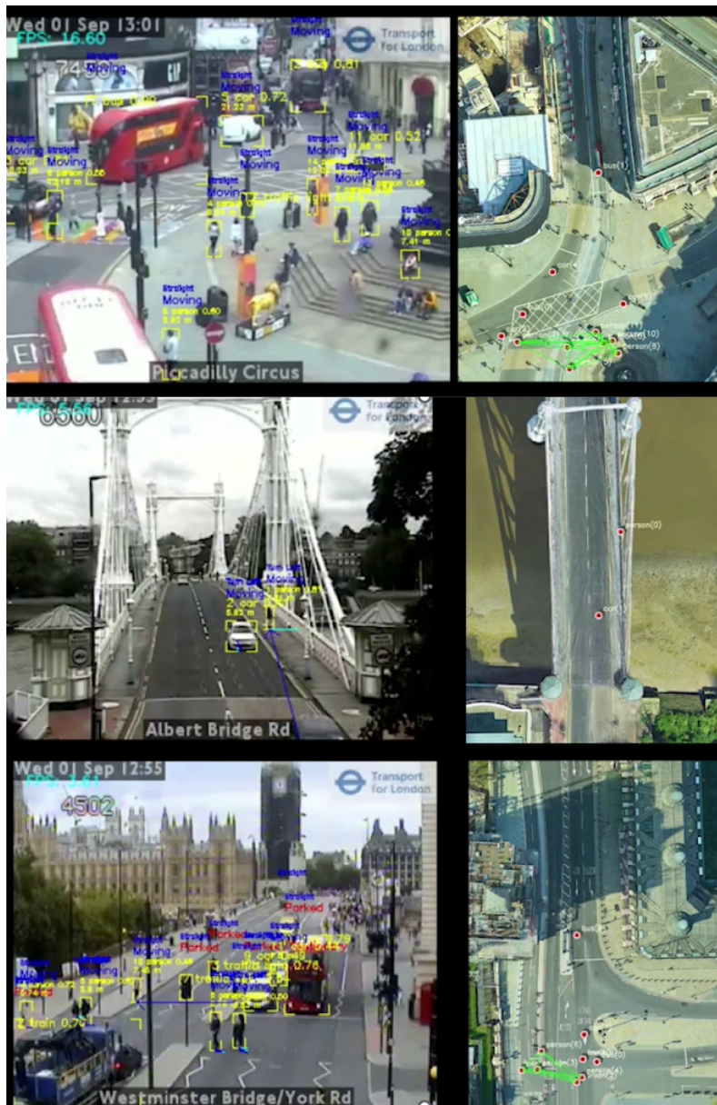
Fig. 1 Examples of different sites of various street layouts and their estimated BEV map on a Google Map.
