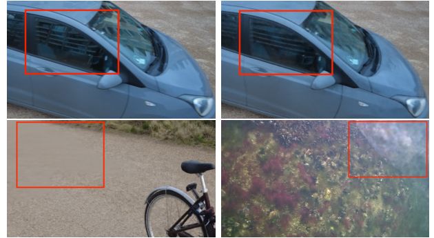
Fig. 12: Examples of NeRF artifacts (enlarged, best seen on screen). Top left: a real image of a reflective surface. Top right: an imprecise rendering in car of the same view as top left. Bottom left: An example of an under-defined pixel patch in bike . Bottom right: An example of a ghost wall in dory1 .
