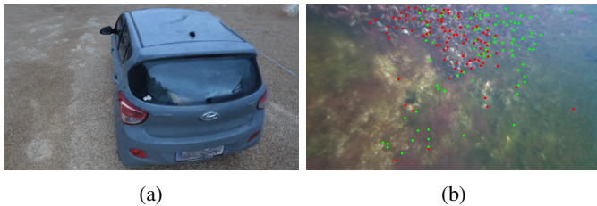
Fig. 9: Examples of inconsistent SUT behaviours: Image (a) transformed by \tau_4 is classified as ImageNet1k class label “trash can” by MobileNet with 0.5285 confidence while having average image metric values (PSNR 15.77, SSIM 0.45, LPIPS 0.72). Image (b) transformed by \tau_4 has a low repeatability score of 0.37 on SuperPoint. The low score is caused by a low agreement of points from the associated real image (green) compared to points found in this image (red). Image (b) has good metric values PSNR 35.12, SSIM 0.70, LPIPS 0.60.
