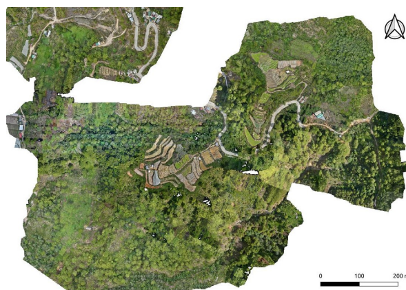
Figure B.2: An excerpt of the Sto. Niño dataset, showing large varieties of vegetation, infrastructure, and image quality. The native resolution of around 2cm/px remains fixed over the entire dataset.
