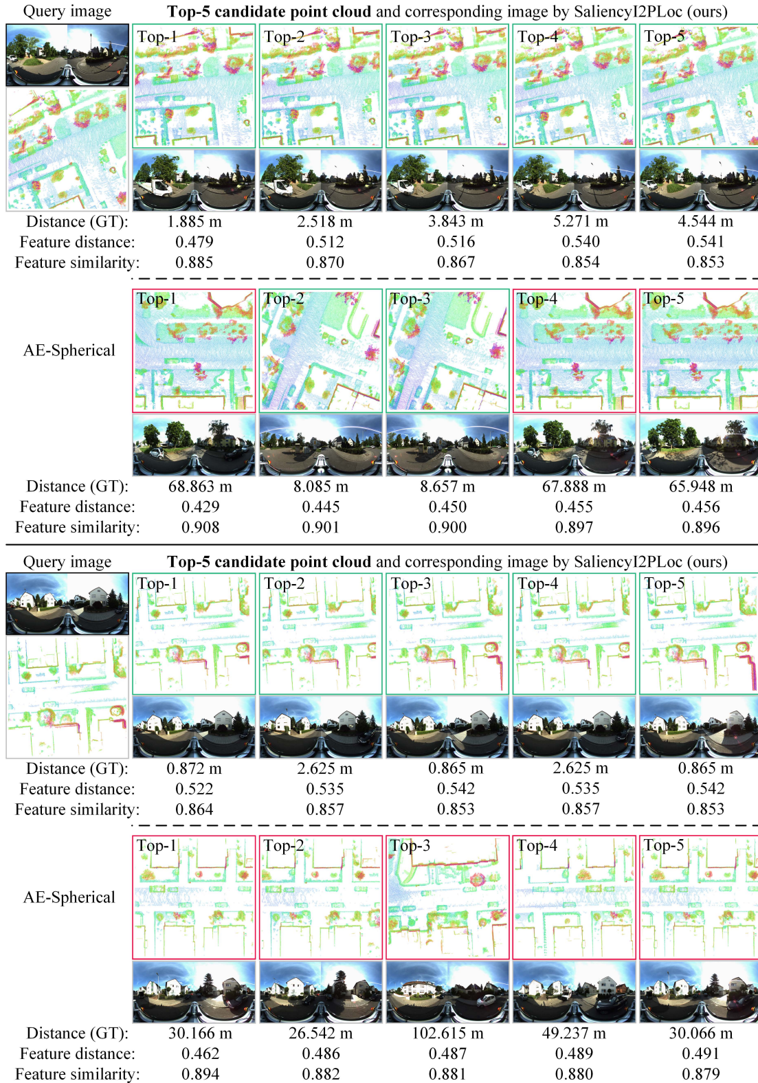
Fig. 13. Visualization of the retrieval results on the KITTI-360 urban scenario evaluation dataset. The green boxes indicate the corrected results, while the red represents the failed ones. The images of each fetched point cloud are displayed for better visualization.
