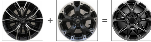
Figure 2: Generating a interpolated combination of two different image sources can create distortion that poses critical challenges to engineering functionality. For example, the distorted spokes are not rotationally symmetrical and hence may distribute force unevenly and affect smooth rolling.
