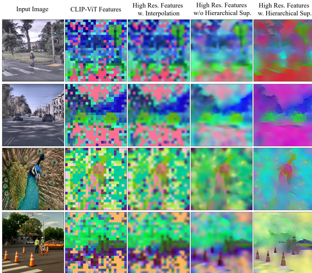
Figure 11: PCA visualization of the up-sampled features by JBU module on nature scene. With hierarchical supervision, the high-resolution features ( 8\times ) could clearly depict object boundary and text appearance. (Best viewed in color and zoomed in)
