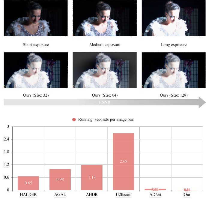
Fig. 1. The top figure shows the results of our method run on a multi-exposure dataset. Size illustrates the scale of the 3D LUT grid, for example, 32 means the size of the grid is 32 \times 32 \times 32 , and the PSNR is gradually increased with the size of the grid. Note that the scale of this grid is editable due to our use of implicit neural representation. The bottom figure shows the average running time comparison over MEFB, a dataset containing 50 image pairs of average size 3 \times 551 \times 707 .
