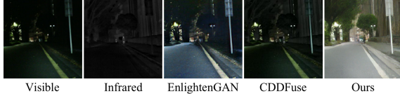
Figure 1. An existing low-light enhancement method EnlightenGAN [20] fails to effectively enhance the image background where most information is obliterated by darkness. The visible and infrared image fusion method CDDFuse [56] reveals the outlines of people and buildings, however, the overall image remains low-luminosity and the region complemented by the infrared image remains sketchy.
