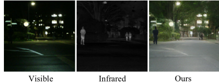
Figure 7. In this instance, although our method enhances the overall perceptual quality and reveals the targets hidden in darkness, the ground indicator unique to the visible image is weakened in the output.
