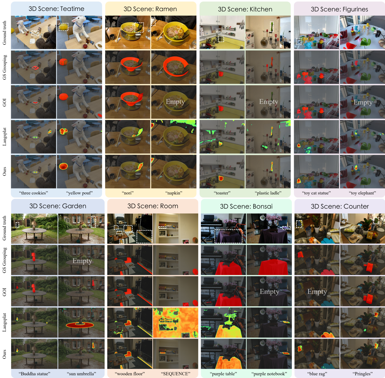
Figure 8. The relevance visualization results for open-vocabulary queries. Each row from top to bottom represents Ground Truth, Gaussian Grouping, GOI, Langsplat, and our method. Below each column is the corresponding input text description.
