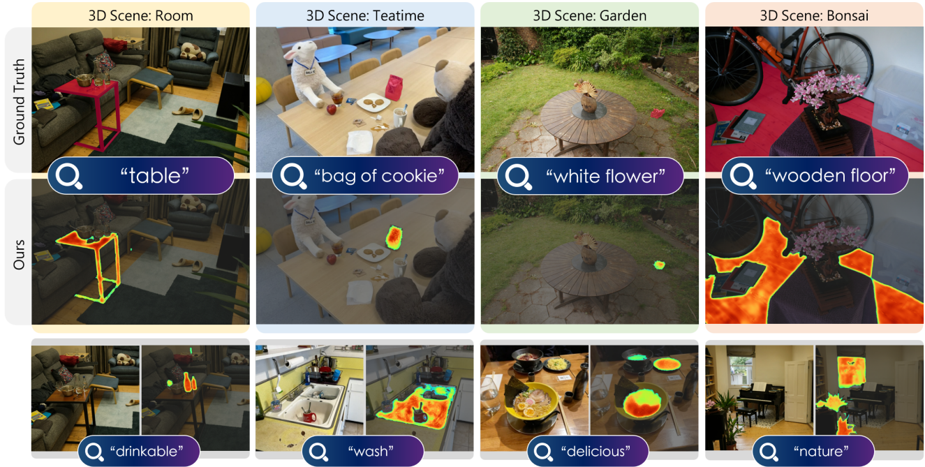
Figure 1. Given multiview images of a scene, GAGS learns a 3D Gaussian field associated with semantic features, which enables accurate open-vocabulary 3D visual grounding in the scene.
