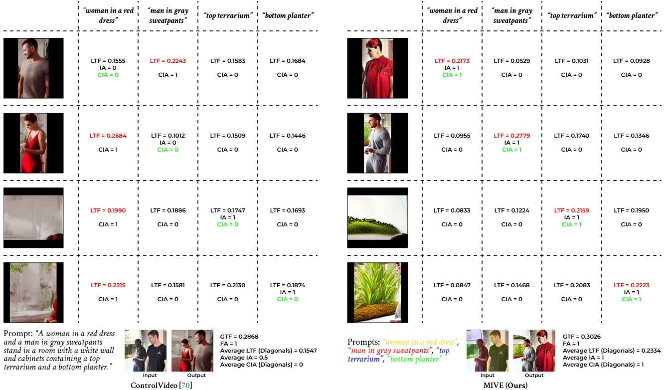
Figure 11. Visualization of the Cross-Instance Accuracy (CIA) Score computation. We calculate the Local Textual Faithfulness (LTF) between each cropped instance and all the instance captions. For each row, we assign 1 to the maximum LTF (shown in red) and 0 to the rest. The CIA Score is calculated as the mean of the diagonal elements (shown in green).
