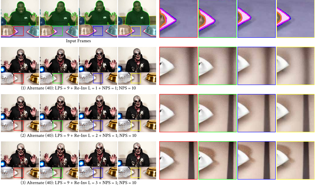
Figure 19. Ablation study on DMS: (c) Ablation on re-inversion step on alternating sampling. Increasing the number of re-inversion steps L in the alternating LPS-NPS steps improves quantitative performance as shown in Tab. 8-(c). We also observe better details with higher values of L . Ultimately, we set L = 3 for the re-inversion in the alternating LPS-NPS stage.
