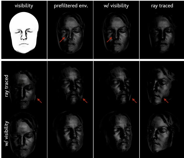
Figure 6. Comparing the specular renders from ray tracing and a pre-filtered environment map. Our proposed view-dependent specular visibility term correctly masks out the unrealistic highlights on the side of the nose, resembling the ray traced results, while produces smoother renders.
