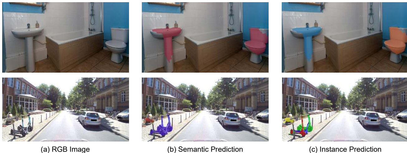
Fig. 6. Qualitative results of our approach, Con2MAV, on open-set panoptic segmentation on COCO (top row), and PANIC (bottom row). The prediction mask is overlaid to the input RGB for clarity. In the semantic prediction, the colored area indicates the anomalous region. In the instance prediction, different colors correspond to different instance ids.
