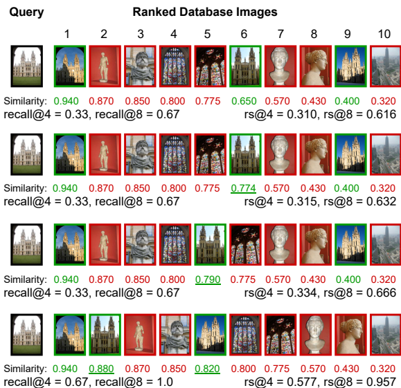
Fig. 2 A comparison between recall@k and rs@k, the proposed differentiable recall@k surrogate. Examples show a query, the ranked database images sorted according to the similarity and the corresponding values for recall@k and rs@k and their dependence on similarity score change. Note that the values of recall@k and rs@k are close. Changes to similarity and ranking in some cases may not affect the original recall@k but can affect the surrogate, with the latter having a more significant impact than the former. Similarity values of all negatives are fixed for ease of understanding. The similarity values of the positives that were changed in rows 2, 3 and 4 are underlined .
