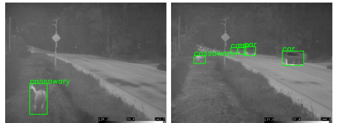
Fig. 8: Demonstrating the system’s detection of a cassowary in thermal imagery from the field trial.
